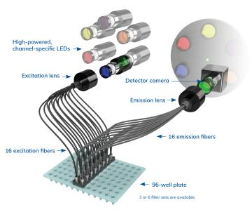
Six targets at once: The Cielo 6 contains 6 high-powered channel-specific excitation and emission light emitting diodes (LEDs) that can distinguish up to 6 different dyes per well without crosstalk or signal leakage. Whereas other instruments are capable of multiplexing 2–3 different dyes, the Cielo 6 detects an entire spectrum of qPCR dyes and chemistries, allowing broad compatibility.
